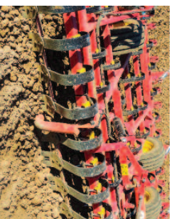
Väderstad's automatic machine adjustment alters implement settings in real time and relative to the current soil conditions.
