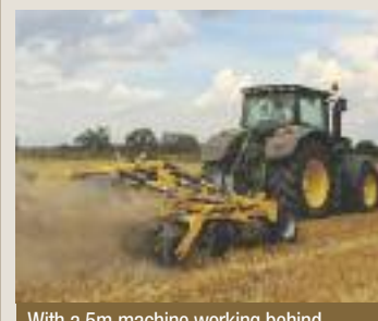
With a 5m machine working behind our 170hp John Deere 6170R we achieved a workrate of 7.3ha/hr using about 5.0l/ha of diesel.
